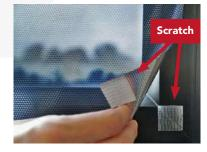
Apply scratch pads to the corners and edges of the film.
